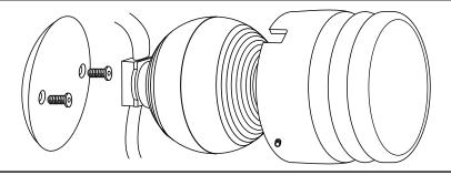
(a). Place the required Globe into the Front Facade housing from the rear and align the cable into the two slots either side.
