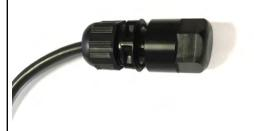
(a). Once the lights are tuned and correct, replace the End of Line Resistor Black cap. Ensure a tight fit for a waterproof seal.
