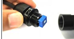
(a). Once the system is powered up and the DMX 512 data transmission is available the end of line units will need setting.Only perform this operation if the installation is flickering and not responding to the 512 DMX data transmission correctly.Remove the Black Cap.
